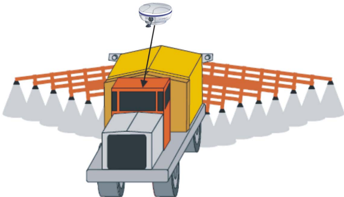
GPS 1500 placement on a vehicle
