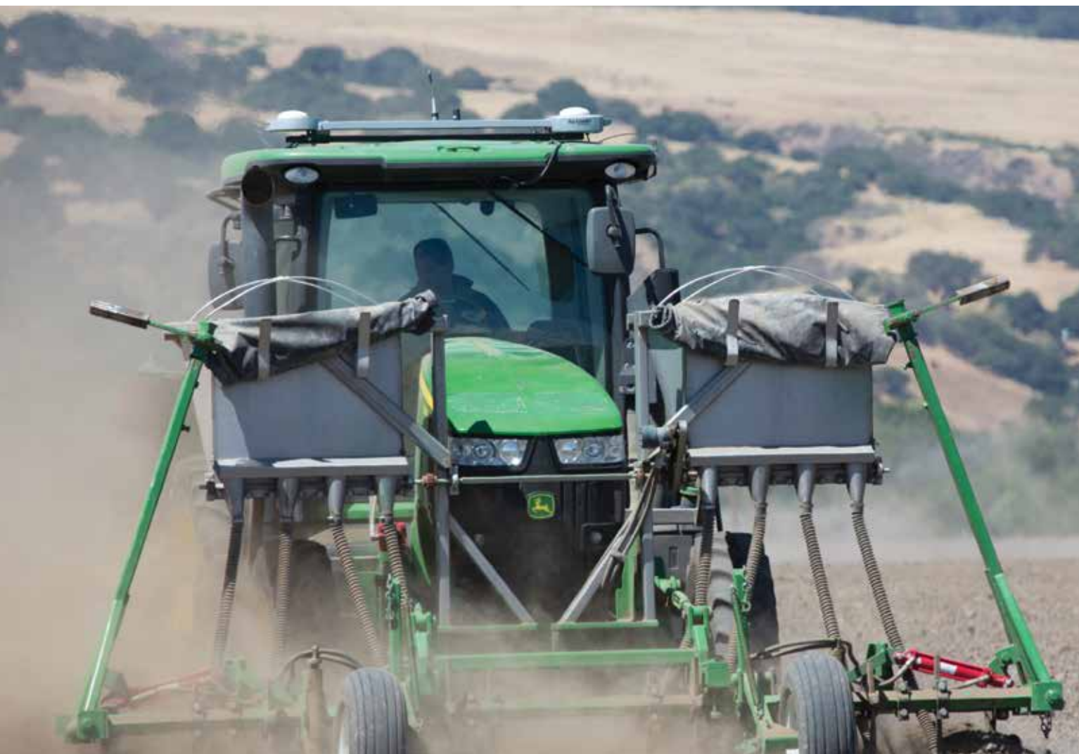
Ag Leader's ParaDyme®, automated steering system, is heavily used in specialty crop production in California due to its accuracy at low speeds.
