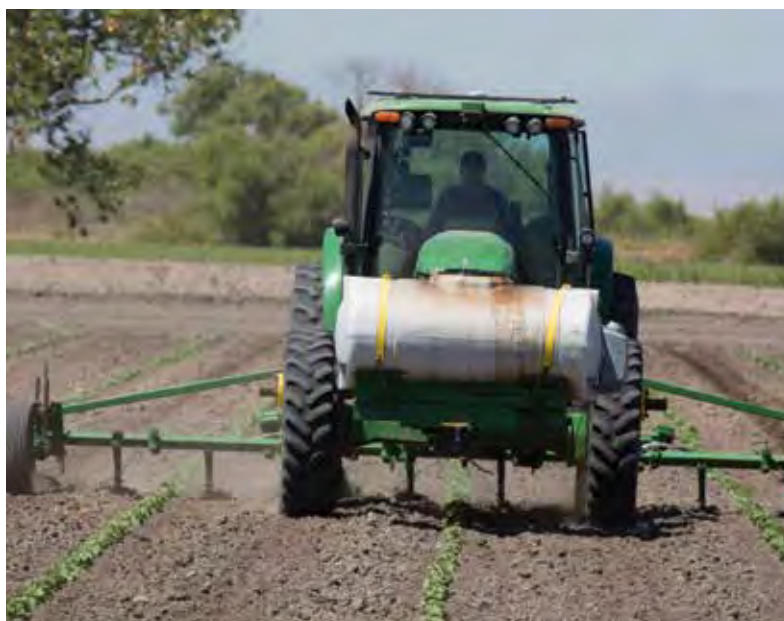
A grower in the Central Valley uses Ag Leader's GPS 1500 and DirectCommand™ System to apply liquid fertilizer to a field of melons.
