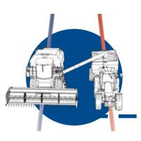
CartACE uses autosteer technology already within the operation to simplify the grain cart operators job. When it's time to unload, the grain cart engages with the press of a button and automatically steers on a line directly under the combine's auger. Autosteer takes over steering to assist operator with accurately unloading on the go.
