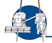
CartACE uses autosteer technology already within the operation to simplify the grain cart operators job. When it's time to unload, the grain cart engages with the press of a button and automatically steers on a line directly under the combine's auger. Autosteer takes over steering to assist operator with accurately unloading on the go.
