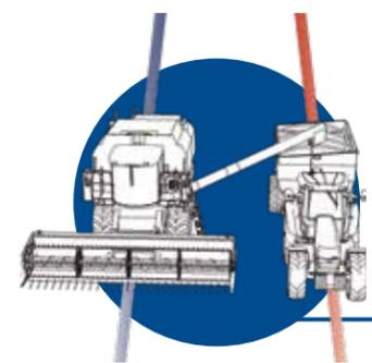
CartACE uses autosteer technology already within the operation to simplify the grain cart operator's job. When it's time to unload, the grain cart engages with the press of a button and automatically steers on a line directly under the combine's auger. Autosteer takes over steering to assist the operator with accurately unloading on the go.
